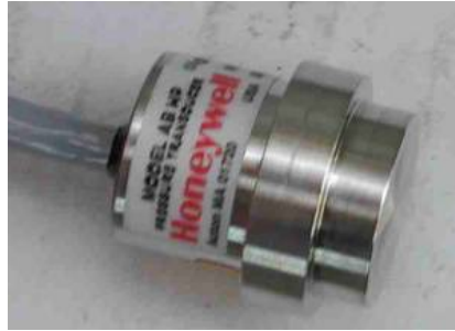
Fig. 2 – Pressure transducer used for measuring lateral pressure
